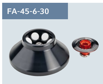
6 × 50 mL conical tube rotor with aerosol-tight QuickLock lid for tubes from 5–50 mL. Max. speed 16,639 × g (11,000 rpm).
